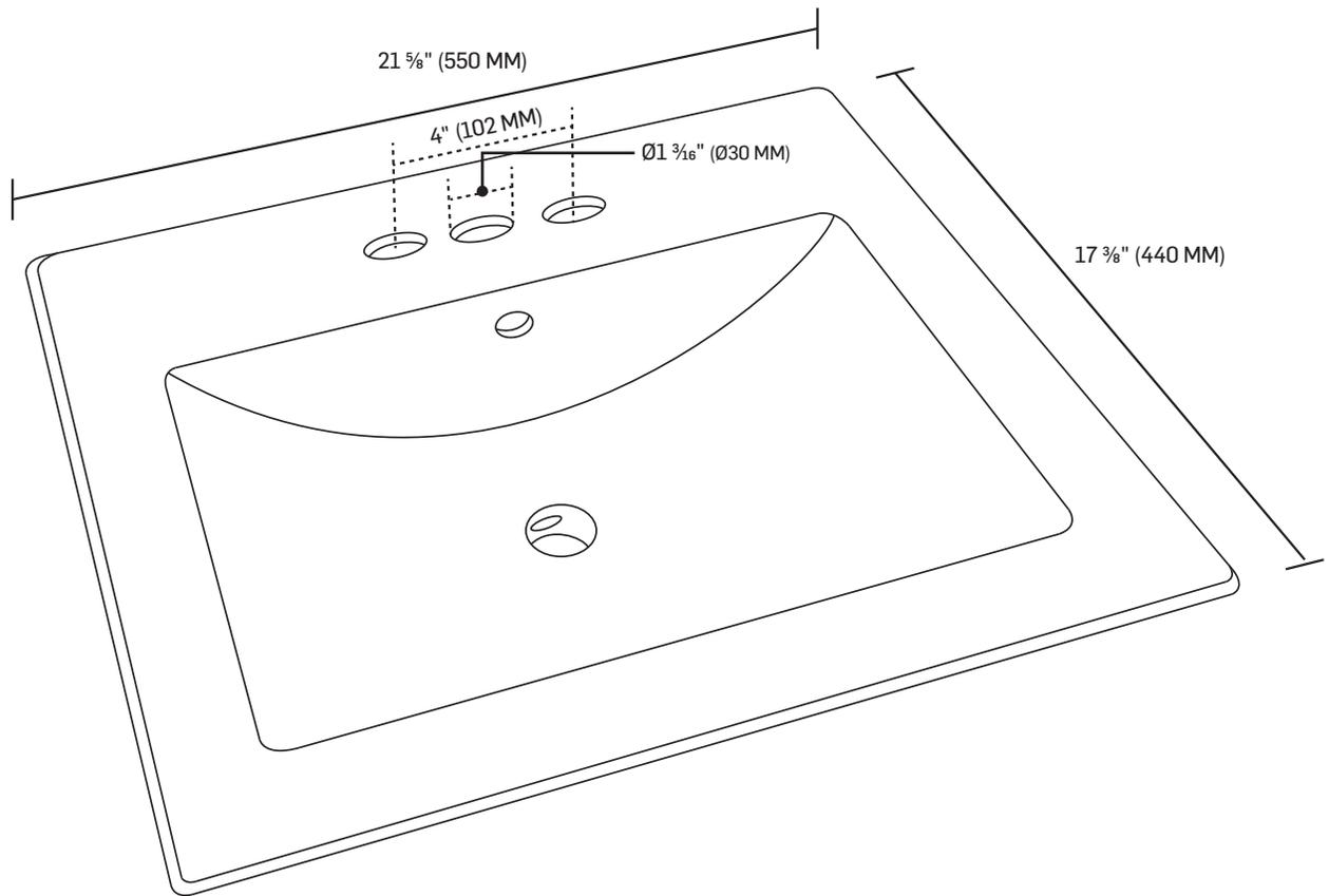
\* TOUTE CES DIMENSIONS SONT APPROXIMATIVES. AFIN D'ASSURER UNE INSTALLATION PARFAITE, LES DIMENSIONS DE LA STRUCTURE DOIVENT ÊTRE VÉRIFIÉES À PARTIR DE L'UNITÉ AVANT L'INSTALLATION.
