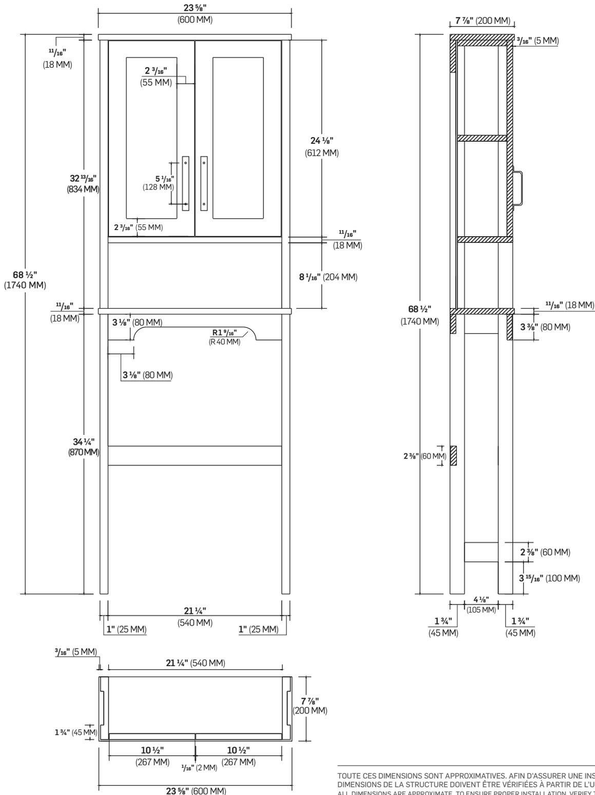
TOUTES CES DIMENSIONS SONT APPROXIMATIVES. AFIN D'ASSURER UNE INSTALLATION PARFAITE, LES DIMENSIONS DE LA STRUCTURE DOIVENT ÊTRE VÉRIFIÉES À PARTIR DE L'UNITÉ AVANT L'INSTALLATION. ALL DIMENSIONS ARE APPROXIMATE. TO ENSURE PROPER INSTALLATION, VERIFY THE PRODUCT DIMENSIONS BEFORE INSTALLATION.
