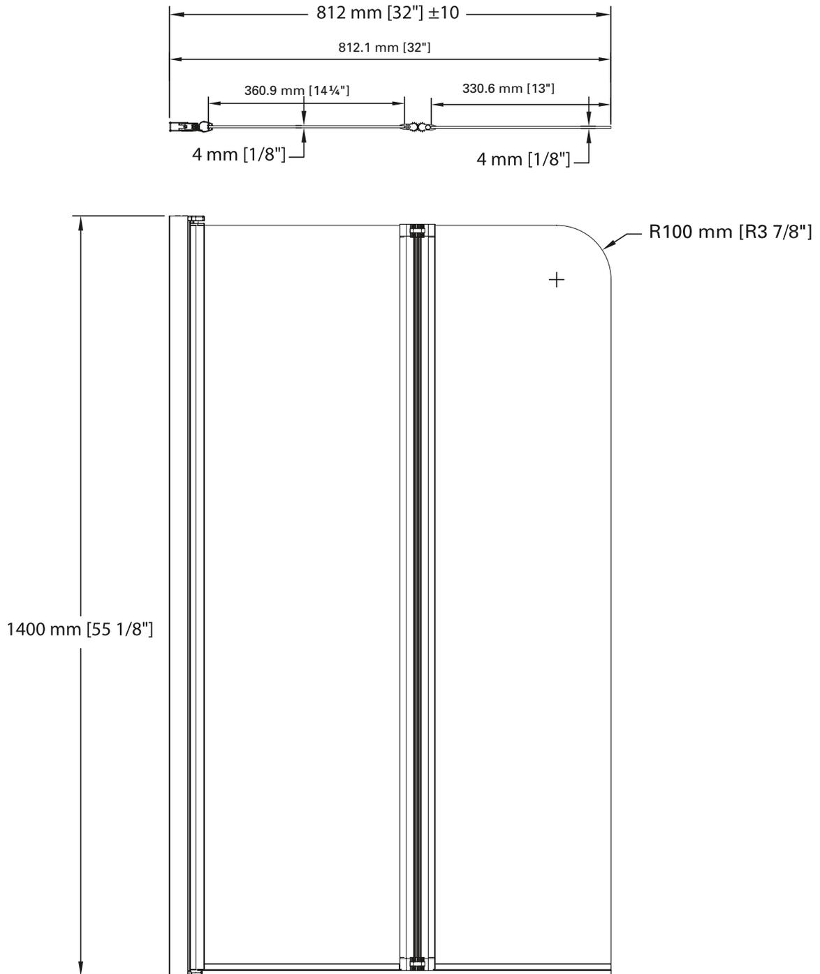
TOUTES CES DIMENSIONS SONT APPROXIMATIVES. AFIN D'ASSURER UNE INSTALLATION PARFAITE, LES DIMENSIONS DE LA STRUCTURE DOIVENT ÊTRE VÉRIFIÉES À PARTIR DE L'UNITÉ AVANT L'INSTALLATION.
