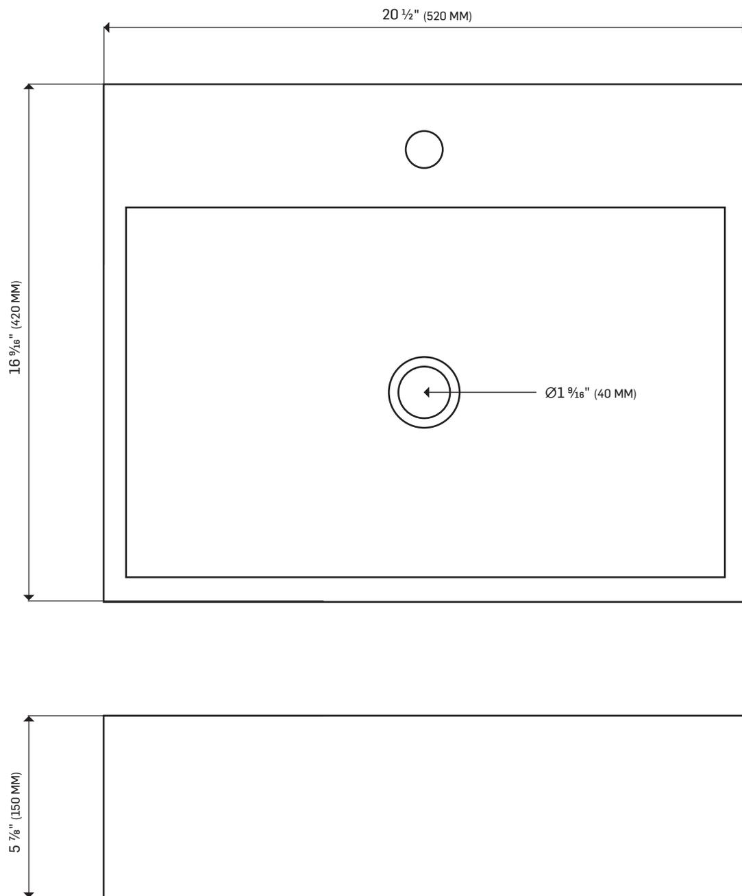
\* TOUTES CES DIMENSIONS SONT À TITRE INDICATIF. AFIN D'ASSURER UNE INSTALLATION PARFAITE, LES DIMENSIONS DE LA STRUCTURE DOIVENT ÊTRE VÉRIFIÉES À PARTIR DE L'UNITÉ AVANT L'INSTALLATION.
