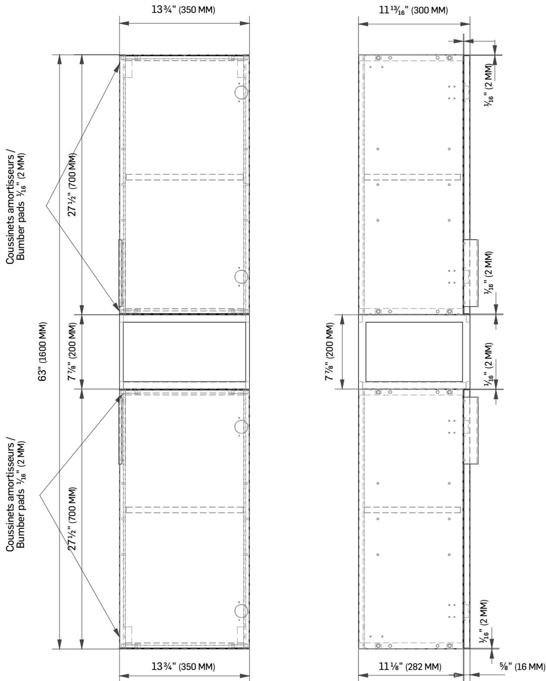
\* TOUTES CES DIMENSIONS SONT APPROXIMATIVES. AFIN D'ASSURER UNE INSTALLATION PARFAITE, LES DIMENSIONS DE LA STRUCTURE DOIVENT ÊTRE VÉRIFIÉES À PARTIR DE L'UNITÉ AVANT L'INSTALLATION.
