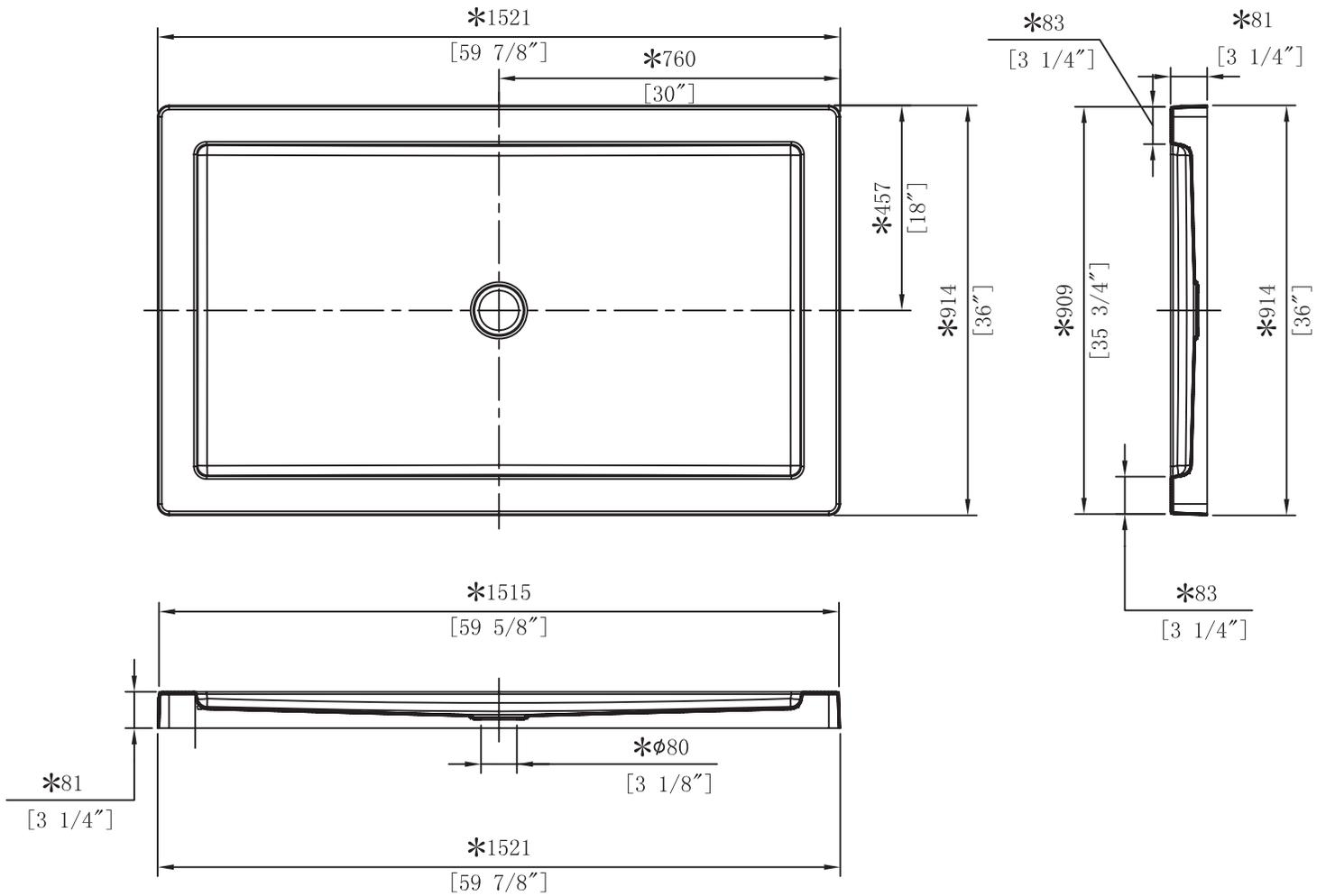
\*TOUTES CES DIMENSIONS SONT APPROXIMATIVES. AFIN D'ASSURER UNE INSTALLATION PARFAITE, LES DIMENSIONS DE LA STRUCTURE DOIVENT ÊTRE VÉRIFIÉES À PARTIR DE L'UNITÉ AVANT L'INSTALLATION.
