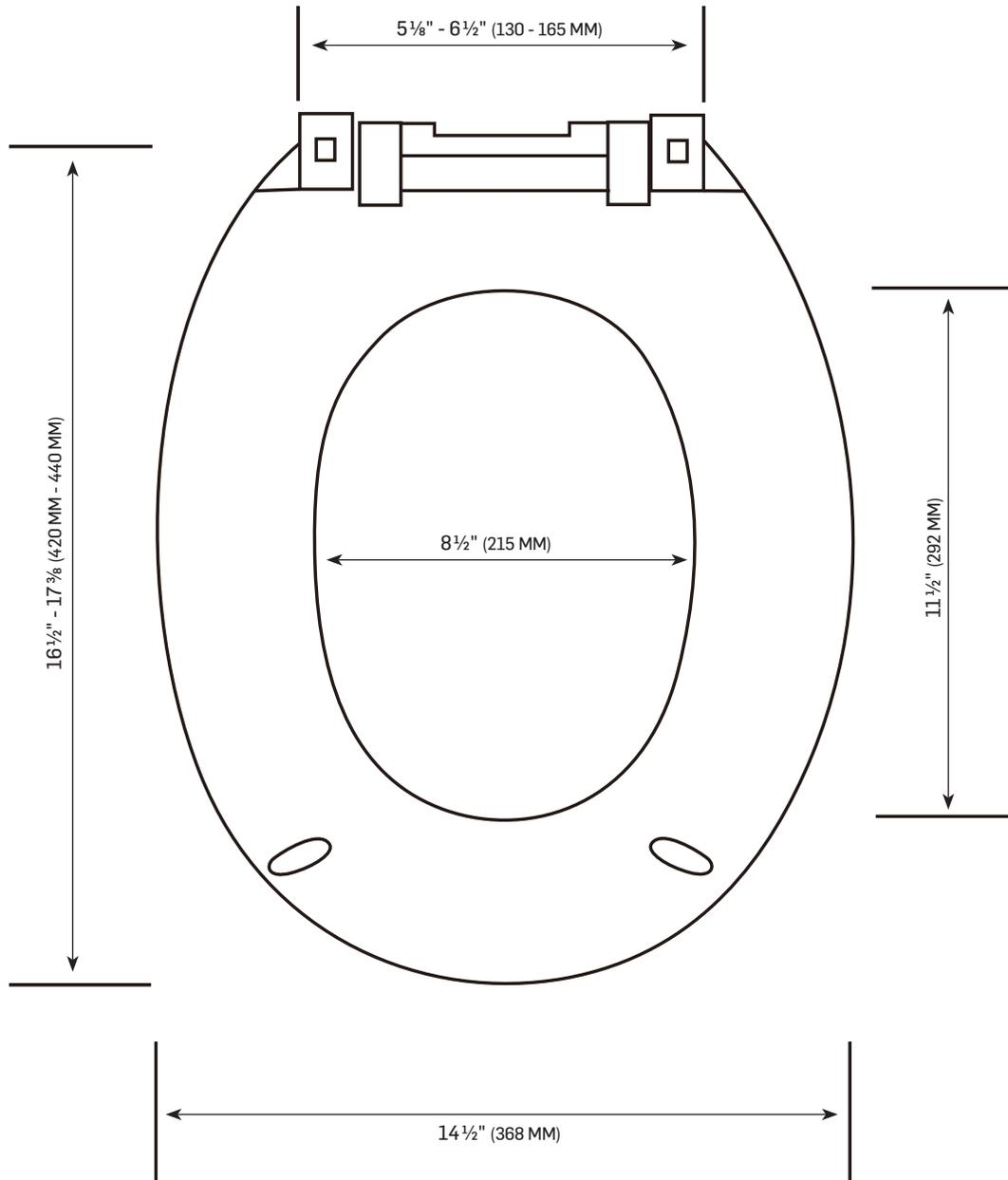
TOUTE CES DIMENSIONS SONT APPROXIMATIVES. AFIN D'ASSURER UNE INSTALLATION PARFAITE, LES DIMENSIONS DE LA STRUCTURE DOIVENT ÊTRE VÉRIFIÉES À PARTIR DE L'UNITÉ AVANT L'INSTALLATION.
