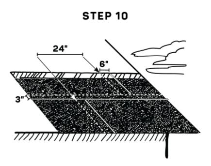
**Valleys and Ridges:** Cut the membrane into 4' (1.2 m) to 6' (1.8 m) lengths. In the valley, start at the low point and work upwards, overlapping each sheet at least 6'' (15 cm). Peel off the release film and center the sheet over the valley or ridge. Drape and press in place working from the center outward toward the edges. Membranes must not be left exposed in an open valley.
