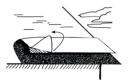
**STEP 9:** Carefully reposition the membrane up onto the deck and press firmly in place. Avoid wrinkles. If more than one course is to be used, the top course should overlap the selvedge tape on the lower course.
