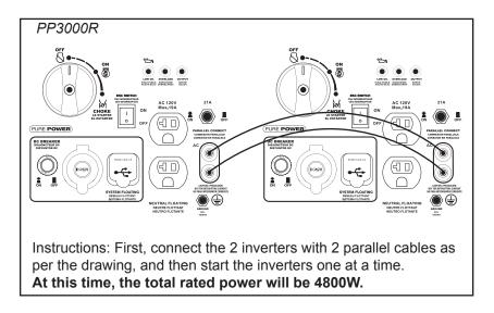
**Note**: Ensure the cables are connected to the inverters correctly. If they are connected incorrectly, the inverters will not output any power and will need to be switched off and then on again after they are correctly connected.
