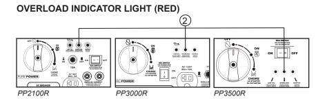
The overload indicator light (2) comes on when an overload of a connected electrical device is detected, the inverter control unit overheats, or the AC output voltage rises. Then, the AC protector will trip, stopping power generation in order to protect the generator and any connected electric devices. The AC pilot light (Green) will go off and the overload indicator light (Red) will stay on, but the engine will not stop running.
