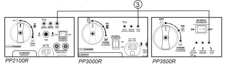
The AC pilot light (3) comes on when the engine starts and produces power.
