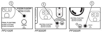
Ground (Earth) terminal (1) connects the earth line to reduce the risk of electric shock. When the electric device is grounded, always ground the generator.
