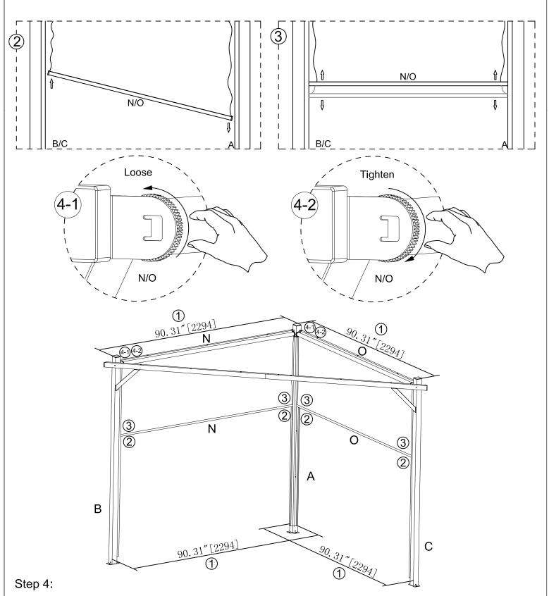
As illustrated, depending on the patio surface, use proper anchoring devices. Anchors are not supplied.
