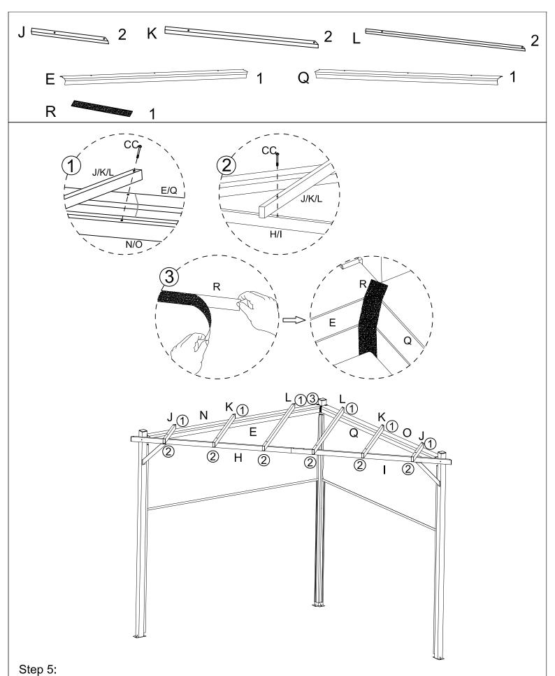
Install the side panel covers (E & Q) onto the crossbars (N & O). Then, fix the roof tubes (J, K & L) onto the crossbars (H/I, N & O) by using the bolts M6x70mm (CC) as shown. Tear the back film of the adhesive tape (R) and stick it in the gap of the side panel cover (E & Q) as shown in fig. 3.
