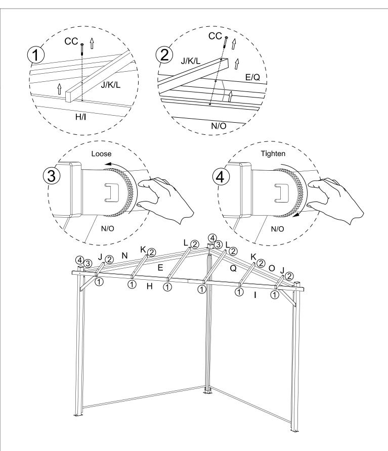
Please note: If you need to readjust the side panel pulling force, remove the bolts M6x70mm (CC), remove the roof tubes (J, K & L), then remove the side panel cover (E or Q). Then, rotate the gear to the appropriate force. Then, reassemble according to the step 5.
