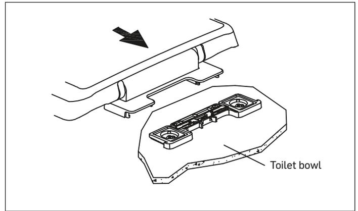
3. Disassembly: Squeeze the hinge pins back in the direction of the arrows. Then slightly push the seat (7) outward.
