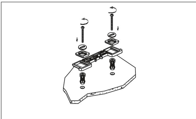
2. Fit the toilet seat onto the hinge seat slots.
