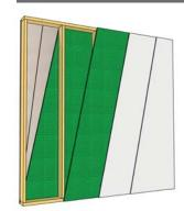
Type X Drywall 15.9 mm (5/8") Type X Drywall 15.9 mm (5/8") **SONOpan** 19 mm (3/4") Wood studs 50.9 mm x 139.7 mm (2 "x 6") at 610 mm (24") c.c. **SONOpan** 19 mm (3/4") Type X Drywall 15.9 mm (5/8") Type X Drywall 15.9 mm (5/8")
