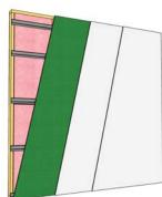
Type X Drywall 15.9 mm (5/8") Wood studs 50.9 mm x 101.6 mm (2" x 4") at 610 mm (24") c.c. R-12 Batt Insulation Resilient channel at 610 mm (24") c.c. **SONOpan** 19 mm (3/4") Type X Drywall 15.9 mm (5/8") Type X Drywall 15.9 mm (5/8")
