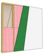
Type X Drywall 15.9 mm (5/8") Type X Drywall 15.9 mm (5/8") Wood studs 50.9 mm x 101.6 mm (2" x 4") at 610 mm (24") c.c. R-12 Batt Insulation 25.4 mm (1") Air space R-12 Batt Insulation Wood studs 50.9 mm x 101.6 mm (2" x 4") at 610 mm (24") c.c. **SONOpan** 19 mm (3/4") Type X Drywall 15.9 mm (5/8")
