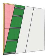
Type X Drywall 15.9 mm (5/8") Wood studs 50.9 mm x 101.6 mm (2" x 4") at 610 mm (24") c.c. R-12 Batt Insulation **SONOpan** 19 mm (3/4") Resilient Channels at 610 mm (24") c.c. Type X Drywall 15.9 mm (5/8") Type X Drywall 15.9 mm (5/8")
