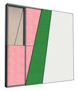
Type X Drywall 15.9 mm (5/8") Type X Drywall 15.9 mm (5/8") Metal studs 50.9 mm x 101.6 mm (2" x 4") at 610 mm (24") c.c. R-12 Batt Insulation
