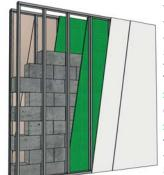
Type X Drywall 15.9 mm (5/8") Type X Drywall 15.9 mm (5/8")
