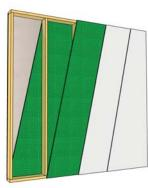
Type X Drywall 15.9 mm (5/8") **SONOpan** 19 mm (3/4") Wood studs 50.9 mm x 139.7 mm (2 "x 6") at 610 mm (24") c.c. **SONOpan** 19 mm (3/4") Type X Drywall 15.9 mm (5/8") Type X Drywall 15.9 mm (5/8")
