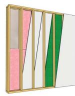
Type X Drywall 15.9 mm (5/8") Wood or Metal studs 50.9 mm x 101.6 mm (2" x 4") at 406 mm (16") c.c. R-12 Batt Insulation Type X Drywall 15.9 mm (5/8") Type X Drywall 15.9 mm (5/8") 25.4 mm (1") Air space R-12 Batt Insulation
