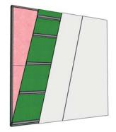
Type X Drywall 15.9 mm (5/8") Metal studs 50.9 mm x 101.6 mm (2" x 4") at 610 mm (24") c.c. R-12 Batt Insulation **SONOpan** 19 mm (3/4") Resilient Channels at 610 mm (24") c.c. Type X Drywall 15.9 mm (5/8") Type X Drywall 15.9 mm (5/8")
