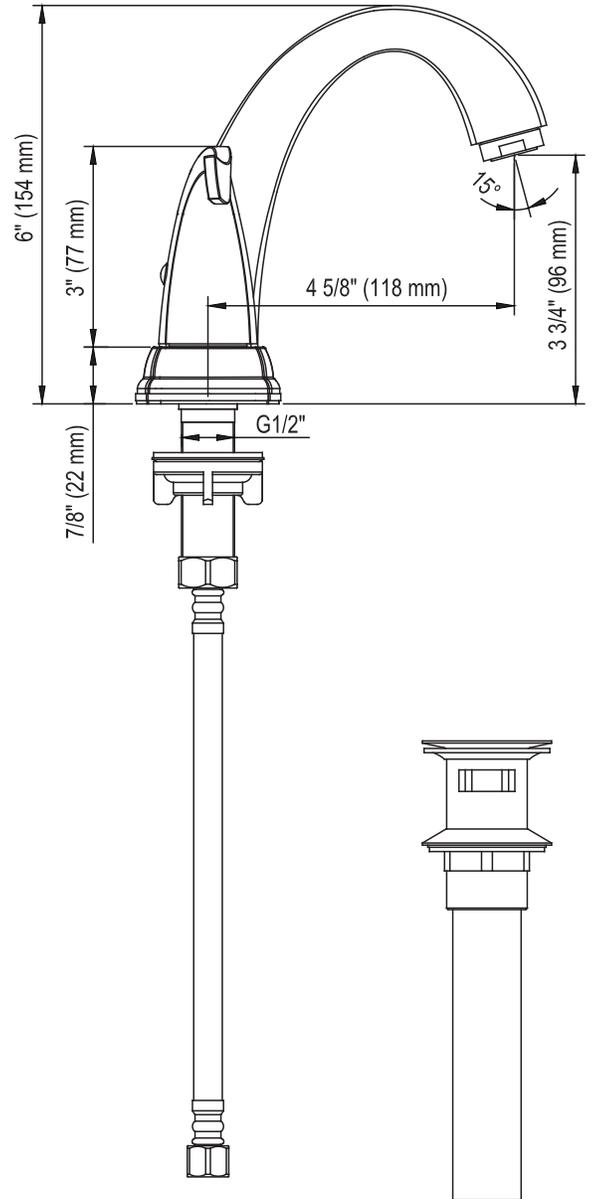
\* TOUTES CES DIMENSIONS SONT APPROXIMATIVES. AFIN D'ASSURER UNE INSTALLATION PARFAITE, LES DIMENSIONS DE LA STRUCTURE DOIVENT ÊTRE VÉRIFIÉES À PARTIR DE L'UNITÉ AVANT L'INSTALLATION.
