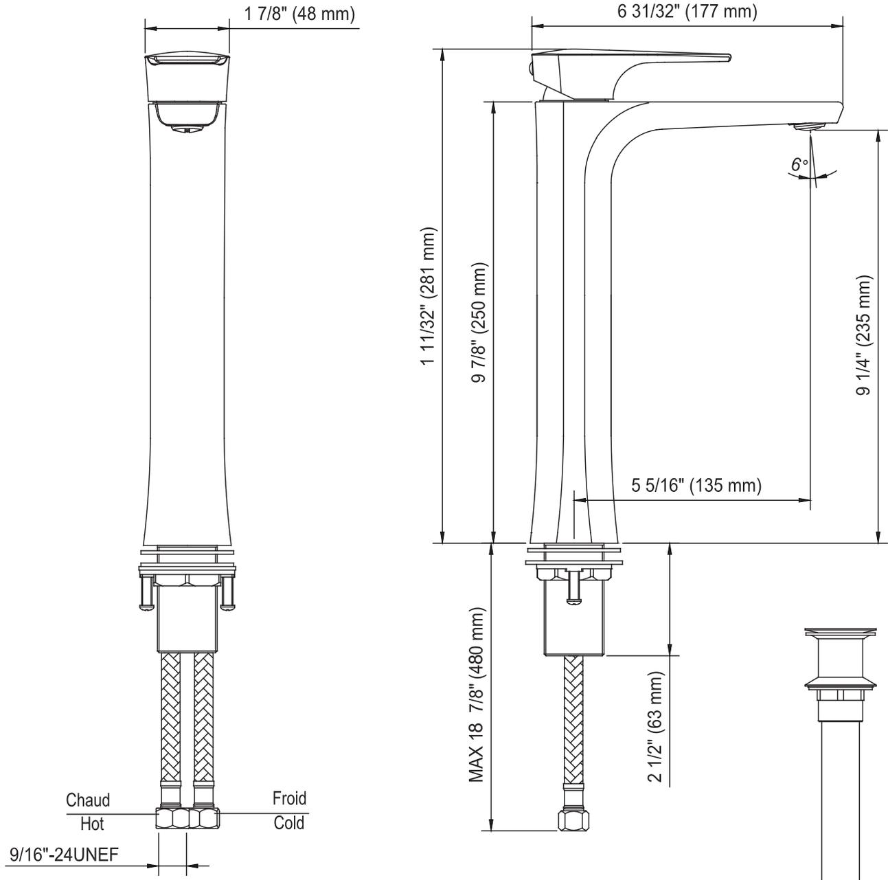
\* TOUTES CES DIMENSIONS SONT APPROXIMATIVES. AFIN D'ASSURER UNE INSTALLATION PARFAITE, LES DIMENSIONS DE LA STRUCTURE DOIVENT ÊTRE VÉRIFIÉES À PARTIR DE L'UNITÉ AVANT L'INSTALLATION.
