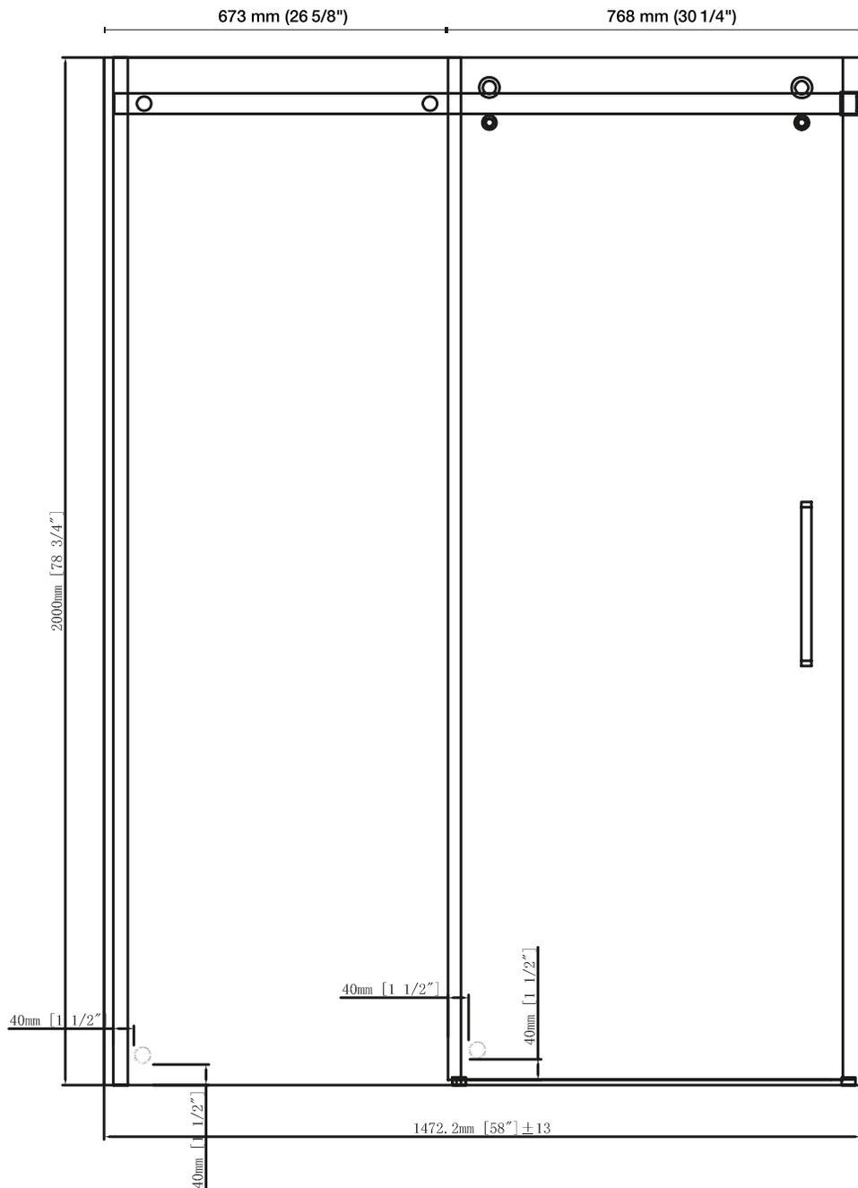
\*TOUTES CES DIMENSIONS SONT APPROXIMATIVES. AFIN D'ASSURER UNE INSTALLATION PARFAITE, LES DIMENSIONS DE LA STRUCTURE DOIVENT ÊTRE VÉRIFIÉES À PARTIR DE L'UNITÉ AVANT L'INSTALLATION.
