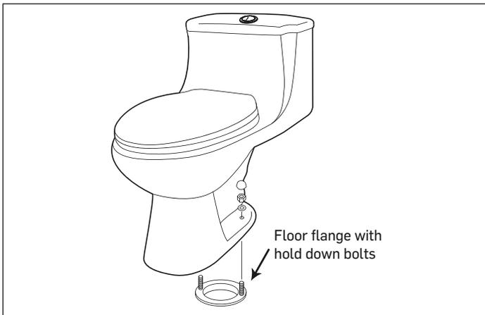
3. Twist and rock bowl as you press it down firmly. As excess wax squeezes out, the bowl will settle into his final position. Install washers and nuts on the holds down bolts and securely tighten, but not tight enough to crack the bowl. Cover the nuts with caps filled with plumber's putty.
