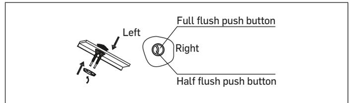
3. Ensure that the full flush button is on the right hand side so that it lines up with 'B' as shown in the diagram.
