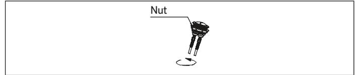
2. Place push button assembly through water tank lid. Fit nut and tighten (do not over-tighten).
