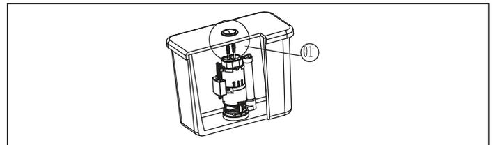
4. The rods for full and half flush can be adjusted up and down by turning the rods clockwise (UP) and counterclockwise (DOWN).
