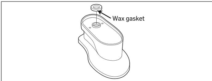
2. Slide two fastening bolts into the slots in the floor flange, packing them with putty to hold them upright, if needed. Lay a rim of plumber's putty around the bowl's flange, pick up the new bowl, turn it right side up and lower it gently over the upright bolts in the floor flange. The wax gasket should meet the flange squarely.
